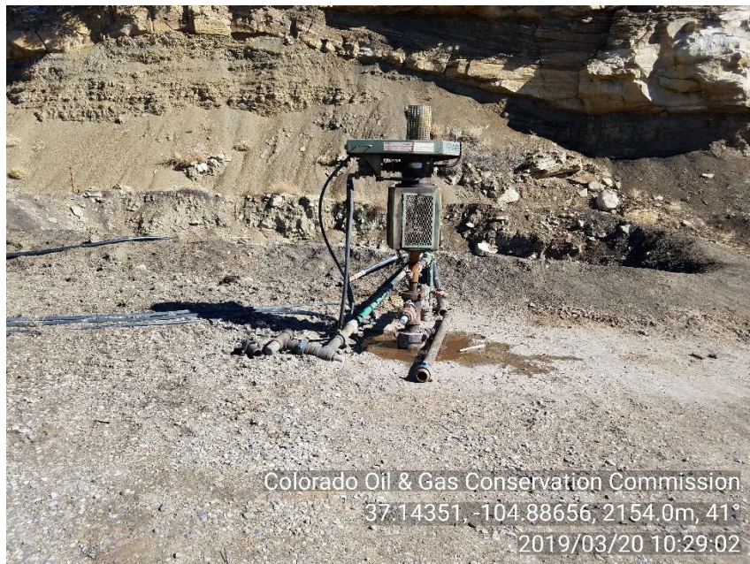
PHOTO 3: UNUSED EQUIPMENT NEXT TO WELLHEAD/ BACKING LEAKING PUMPER ON LOCATION FIXING PACKING LEAKE DURING INSPECTION
