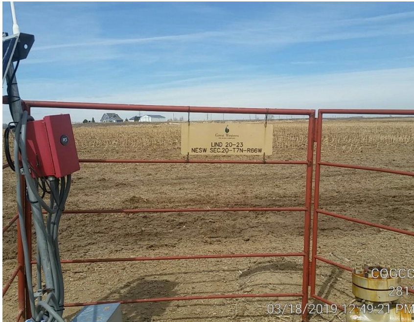
Photo 1 – Wellhead Sign, missing Emergency Contact #
