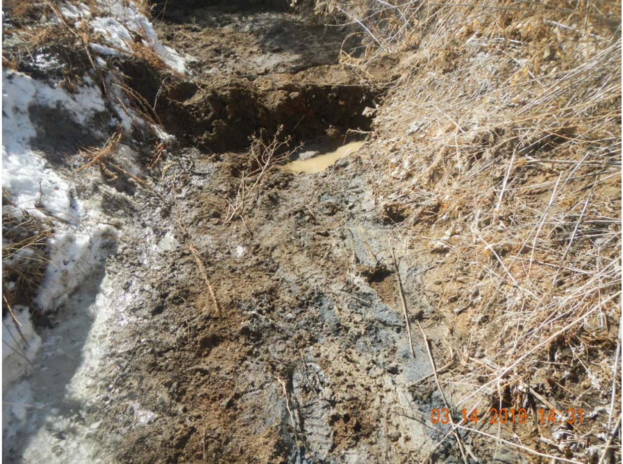
Two Potholes were dug in creek bed, downstream from spill point. One pothole visible here, one approximately five feet below (near shadow)..
