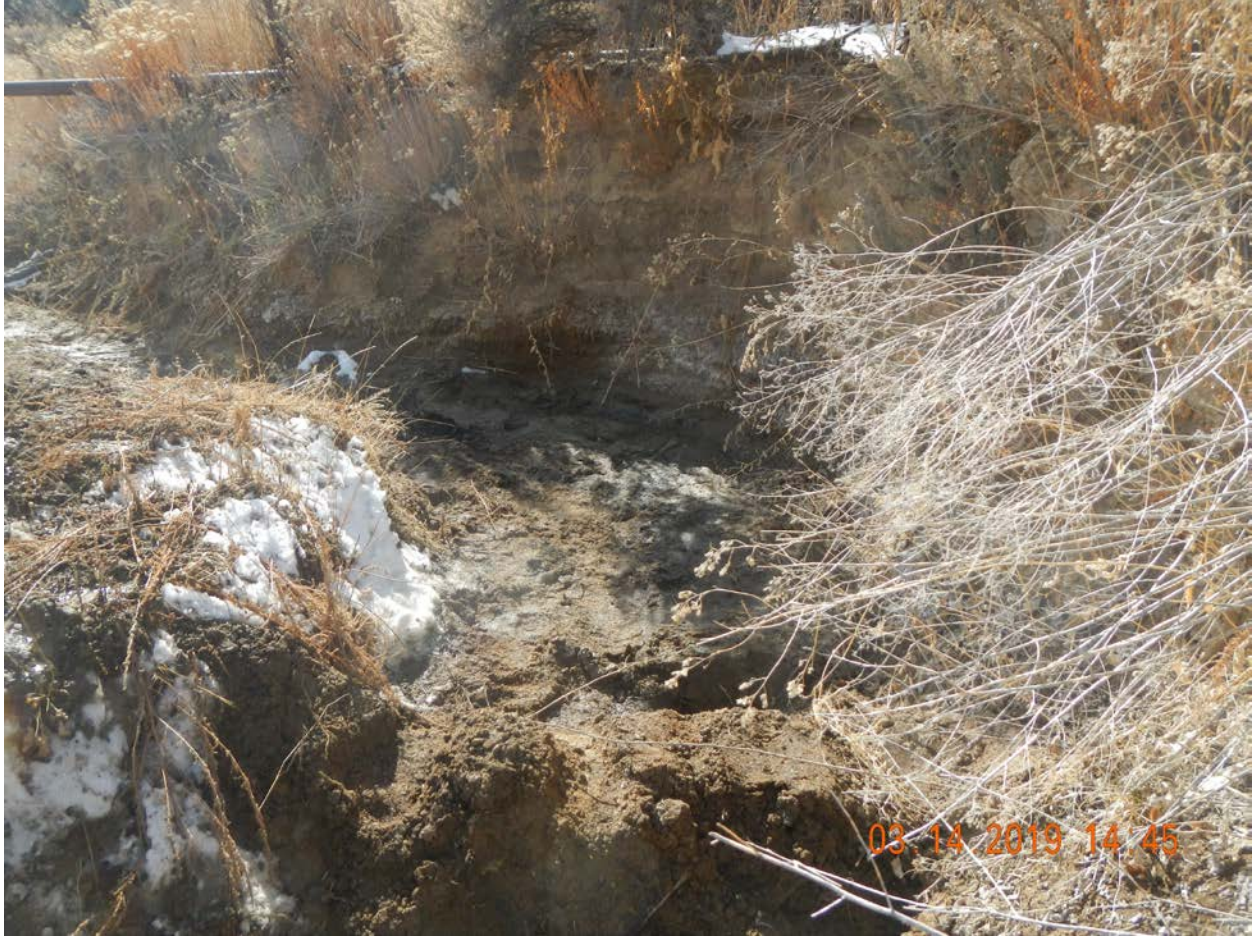
Two Potholes were dug in creek bed, downstream from spill point. This appears to be the end point.
