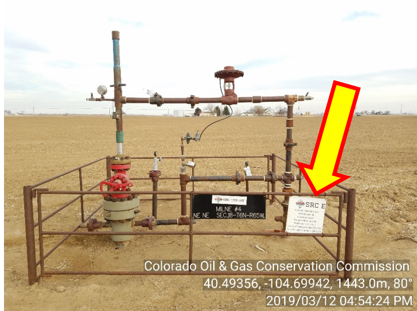
Photo #1 Milne #4 (05-123-12793) Wellsite Shut-In | SI Incorrect Emergency number posted
