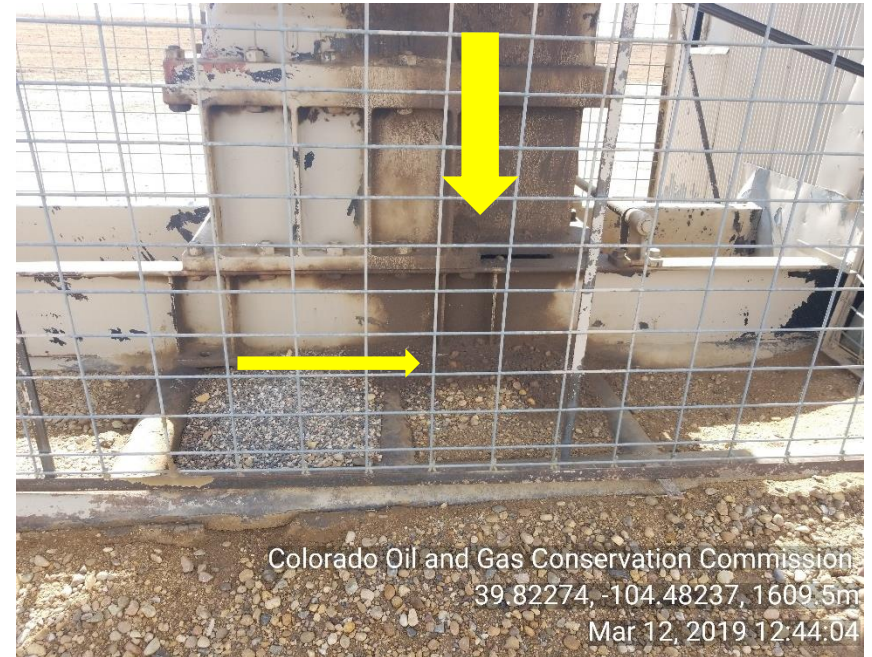
Photo 2 Stained soil and gear box has leak (mechanical issues)
