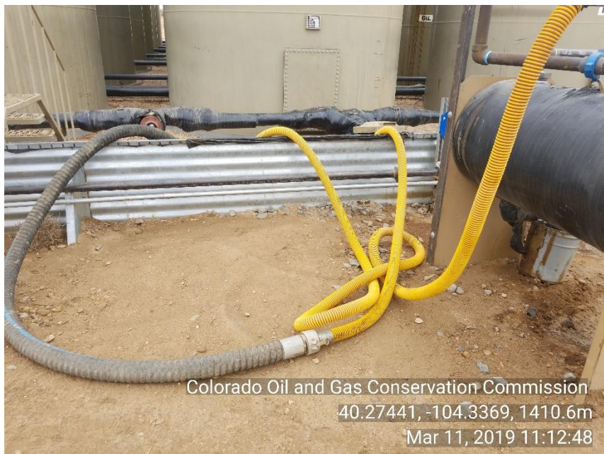
Photo 15 unused equipment hoses for loading out not stored properly and outside containment
