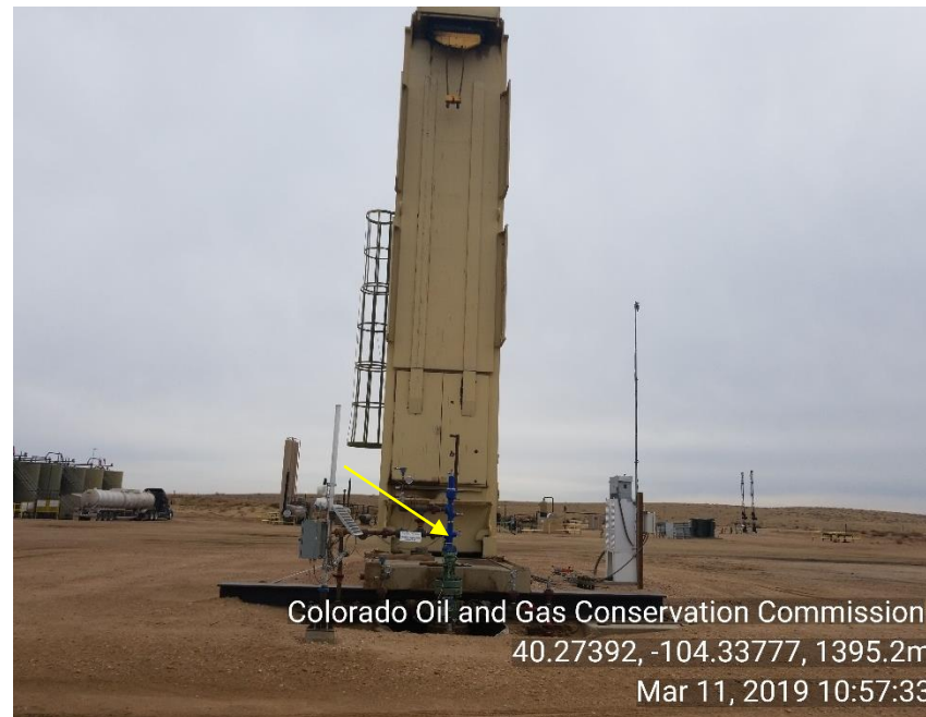
Photo 2 WH/ unused equipment hyd PU not being used WH has Plunger lift.
