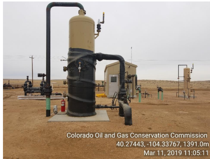
Photo 10 Vert separators and separator building.
