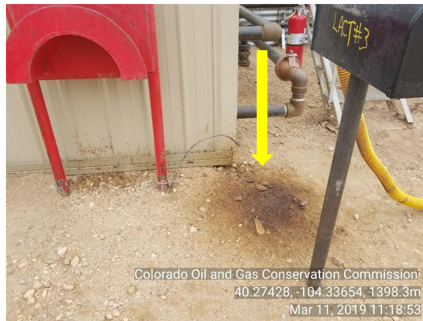
Photo 28 stained soil outside lact bulking out side of crude oil containment
