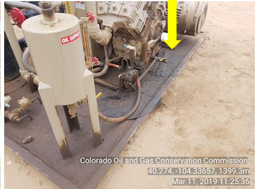
Photo 36 environmental diapers soaked with what appears to be oil hanging off skid
