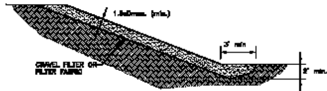
FIGURE R-2 Typical Riprap Slope Protection Detail
