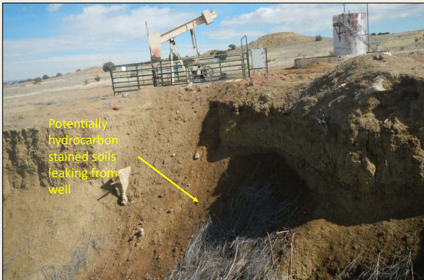
Photo 2. View of the well had from the southwestern edge facing northeastward. Active erosion is visible. Dark soils may indicate oil-stained soils. Location is not stable.
