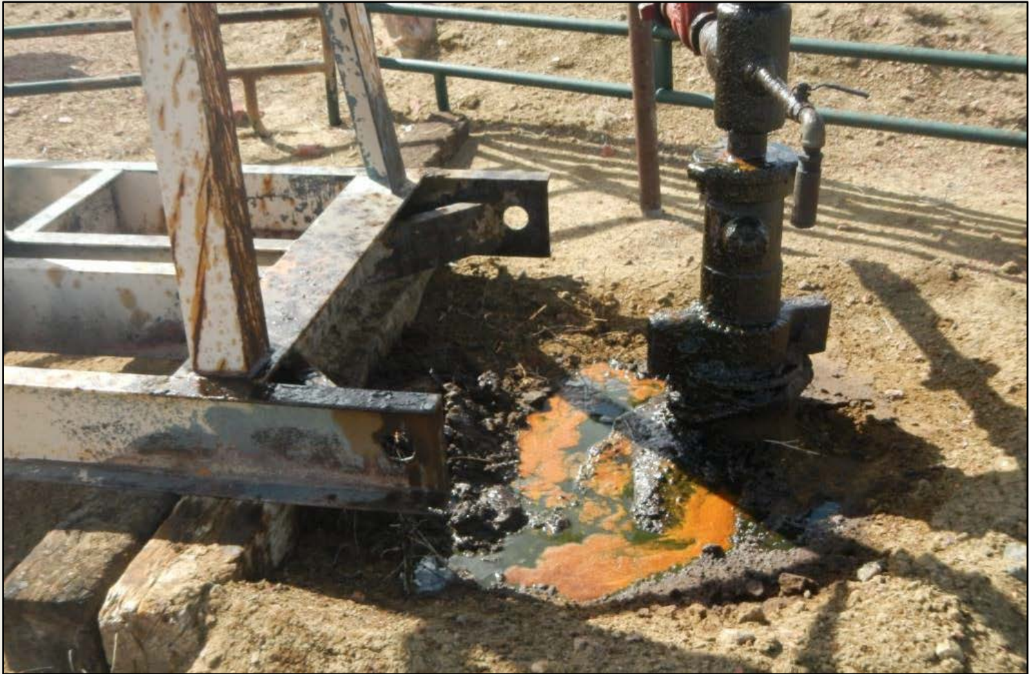
Photo 3. View of hydrocarbon material pooling around wellhead.
