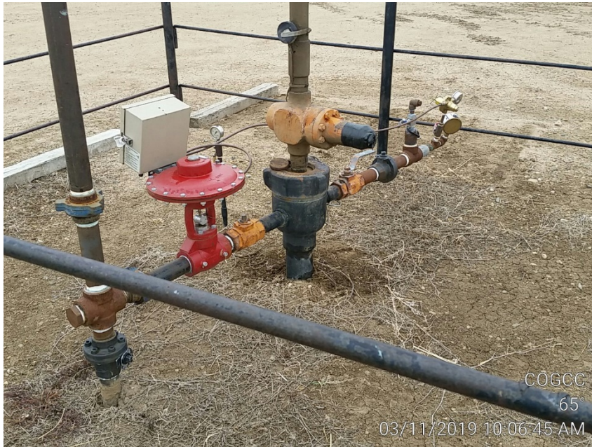
#3 Broken Master Valve Comply W/ 605.d
