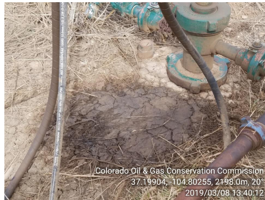
PHOTO 4: IMPACTED SOIL BENEATH SEEPING HYDRAULIC LINES.
