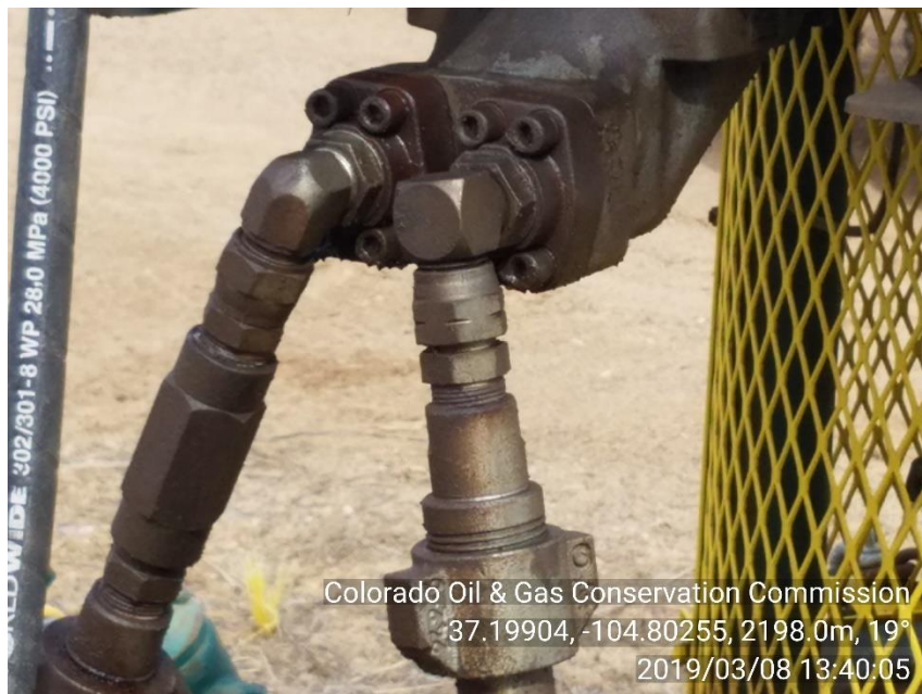
PHOTO 3: HYDRAULIC LINES ARE SEEPING HYDRAULIC FLUID
