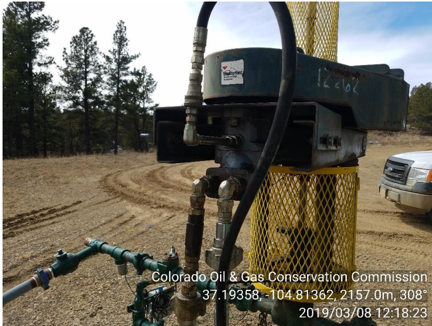
PHOTO 3: I WITNESSED 1" HYDRAULIC LINE DRIP HYDRAULIC FLUID.
