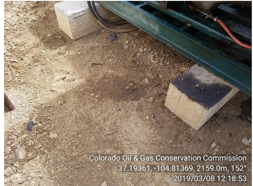
PHOTO 6: IMPACTED SOIL ON NORTH SIDE OF ENGINE SKID. I COULD NOT DETERMINE SOURCE OF LEAK.
