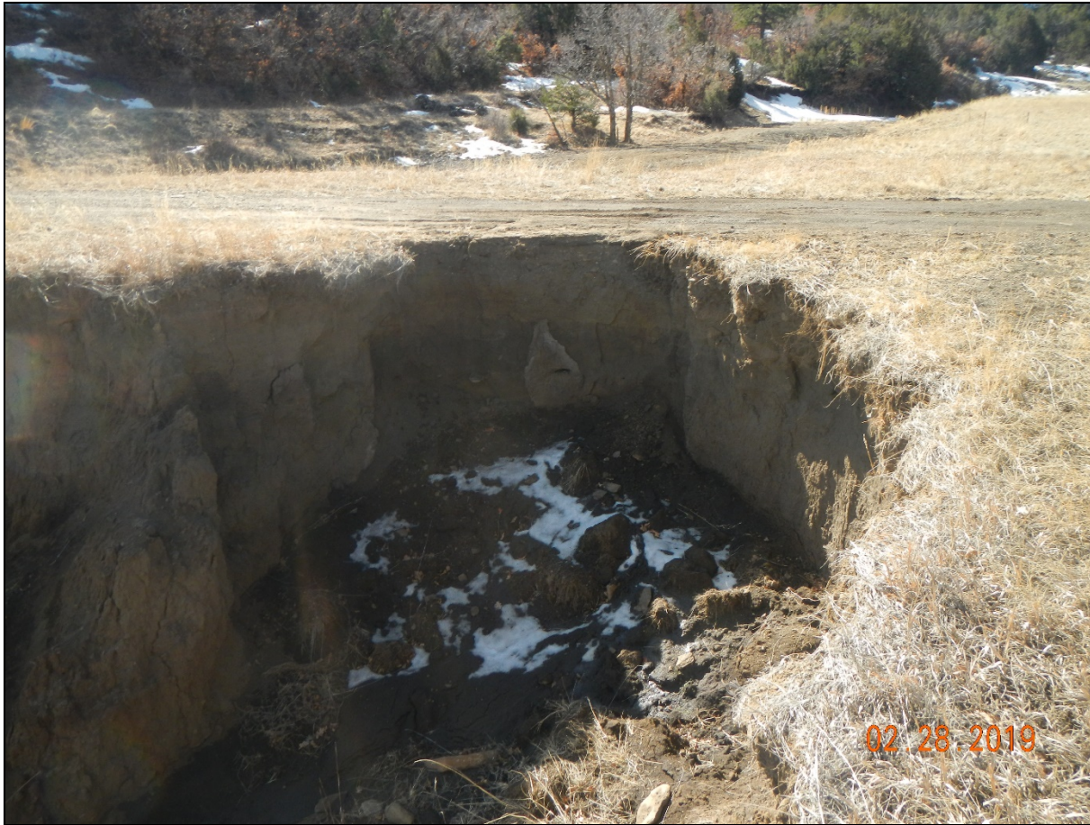
Photo 2. Stormwater appears to flow across the road causing significant erosion.
