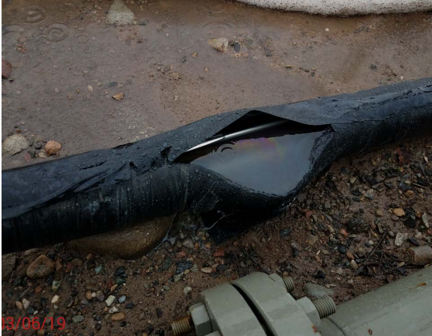
Location Photo #11, Area of the leak.
