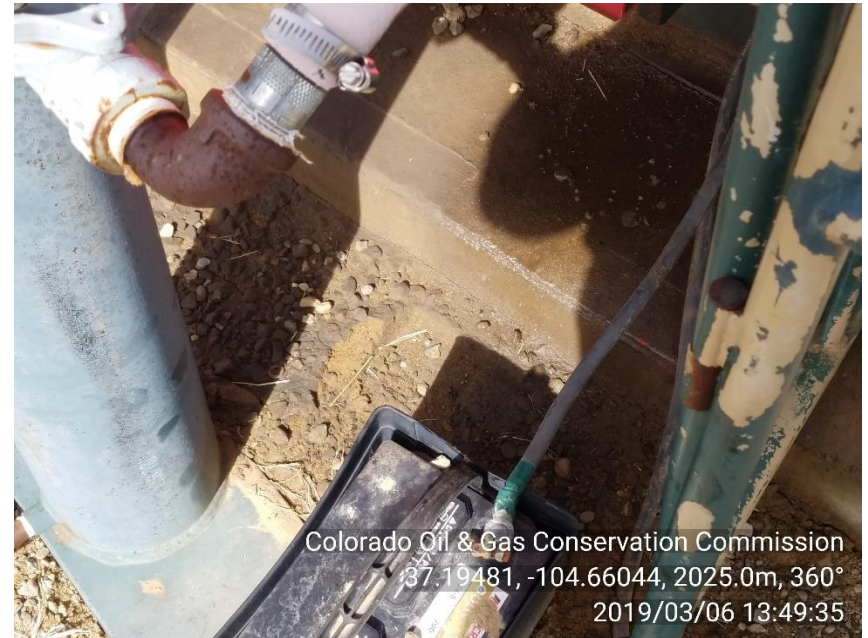
PHOTO 4: IMPACTED SOIL/ OIL APPEARS TO BE LEAKING FROM PUMPJACK MOTOR AND RUNNING ONTO THE GROUND ON SOUTHWEST SIDE OF PUMPJACK
