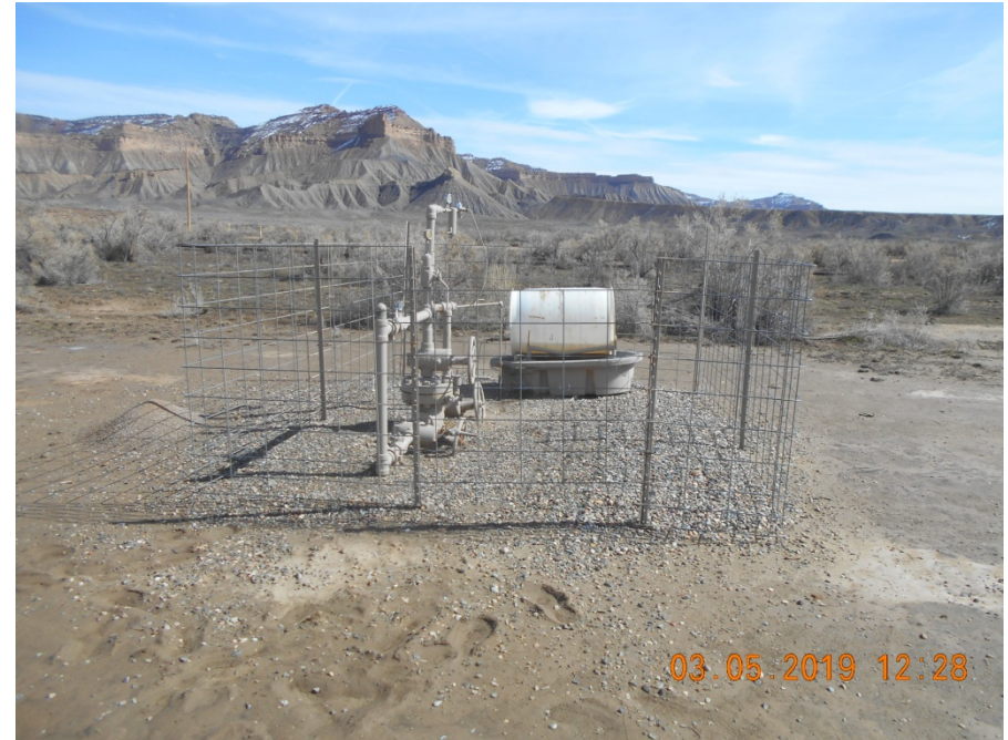
Wellhead with fence. Secondary containment of chemicals.
