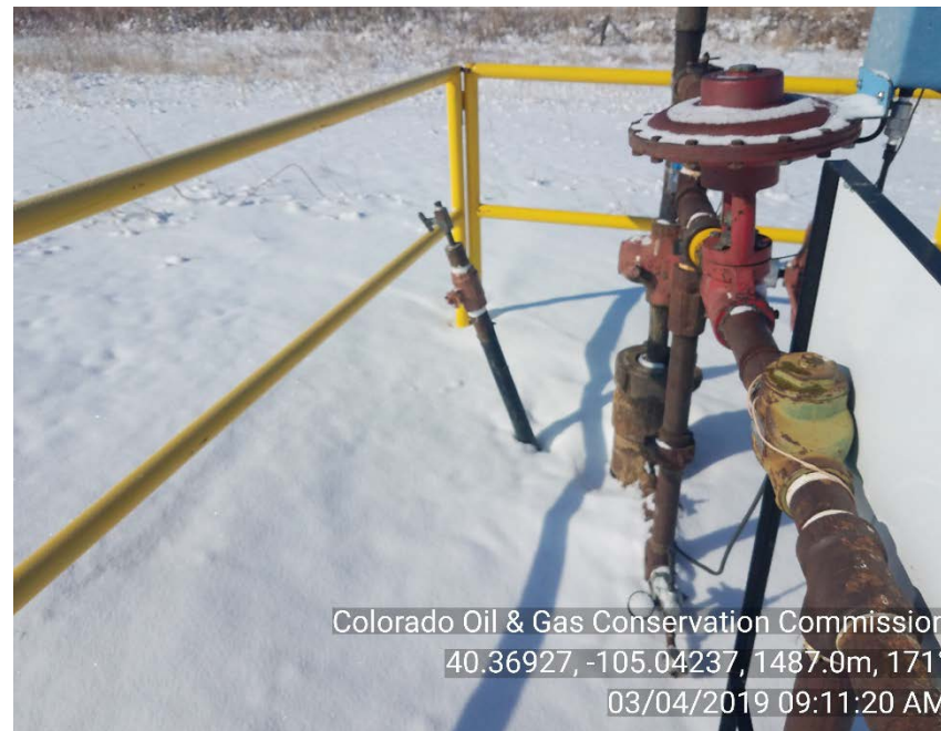
Bradenhead valve on 3/4/2019
