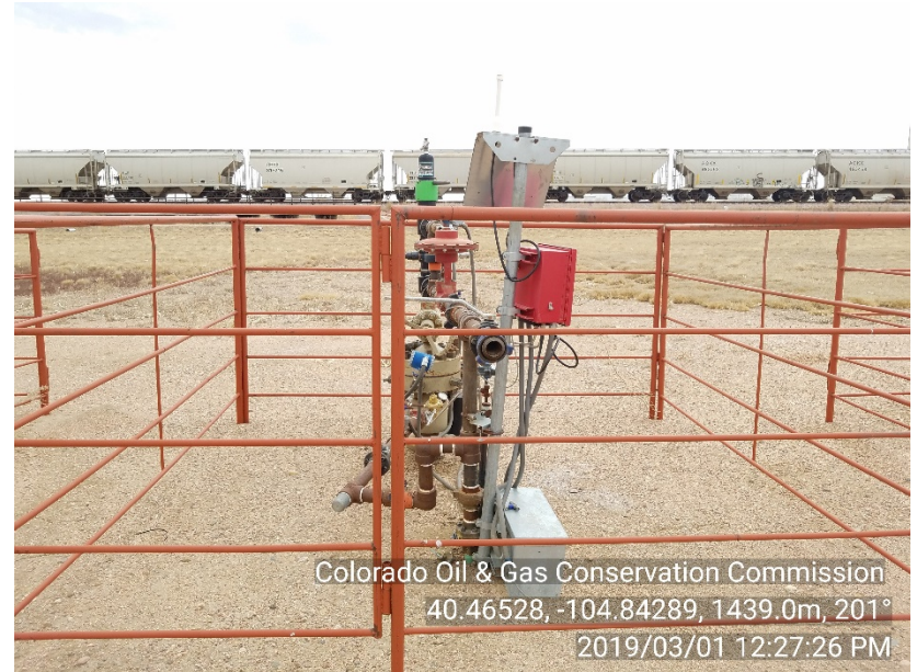
Photo #2 HCW FD 24-35D (05-123-35599) Wellsite Shut-In | SI Sign & Emergency number NOT posted
