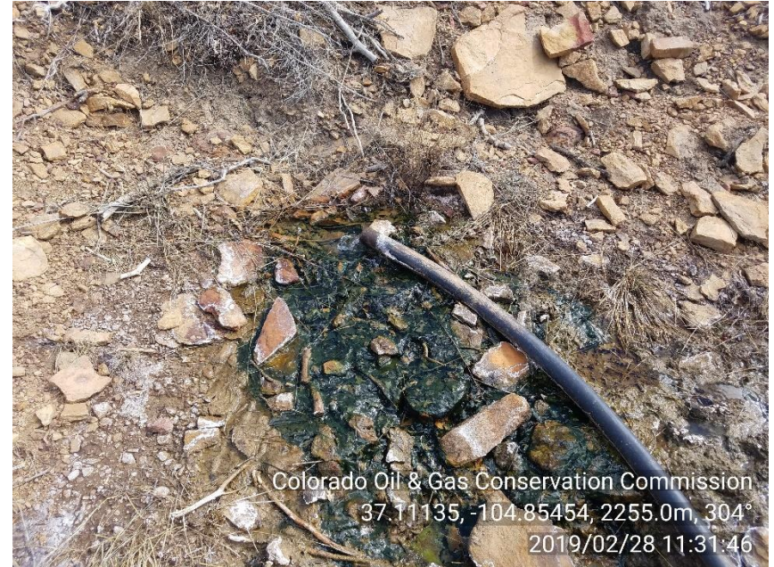
PHOTO 4: PRODUCED WATER DISCHARGE POINT.
