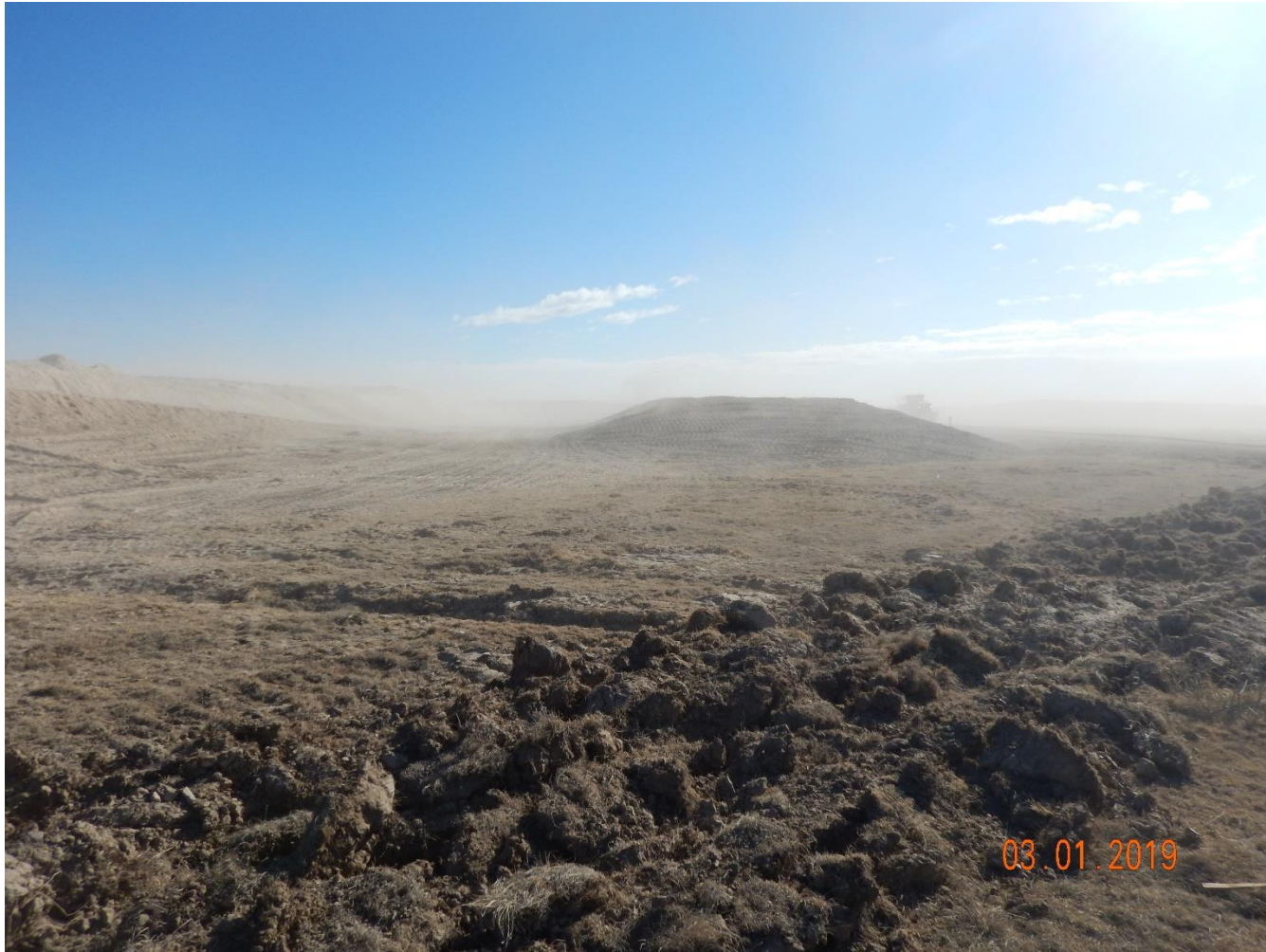
Photo 4: Photo taken from the south end of the location, facing east. Photo shows ongoing wind erosion degradation transporting sediment off of the location and soil stockpiles.
