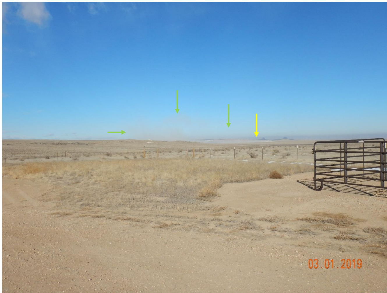
Photo 21: Photo taken from the north end of the Shable LD #21-68HN tank battery (123-36951), facing northwest towards the LD07-01 MULTI construction pad (yellow arrow). The Shable location is ~3 miles from the LD07 pad. Photo shows the dust cloud (green) due to wind erosion transporting sediment from the LD07 pad. Dust cloud appears to be several hundred feet in the area and is visible several miles from the location.
