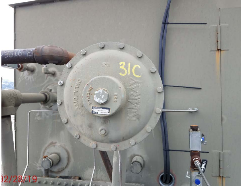
Location Photo #10, Leaking fitting on unit 31C.
