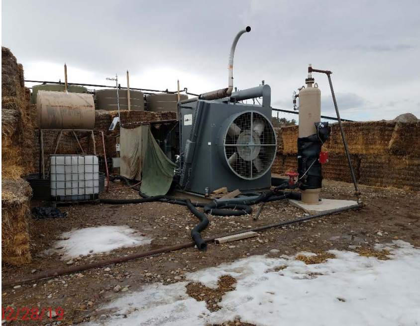
Location Photo #5, Temporary compressor for gas lift operation.
