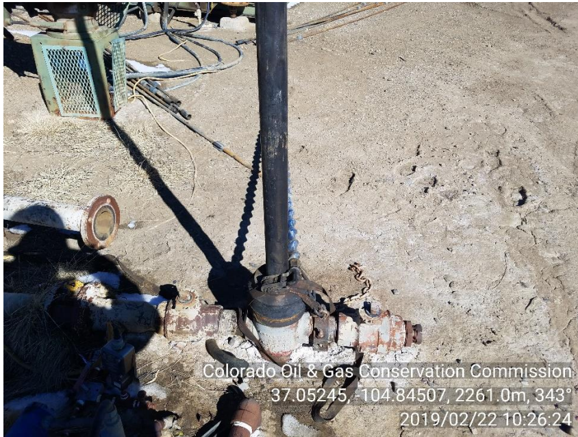
PHOTO 3: WELLHEAD IS IN DISREPAIR AND IS HELD TOGETHER WITH A RATCHET STRAP. I CAN HEAR PRESSURE ESCAPING FROM WELLHEAD.
