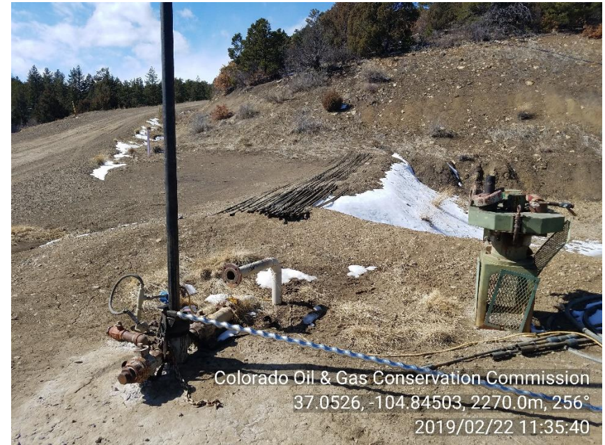
PHOTO 4: UNUSED EQUIPMENT ON LOCATION (UNUDED RISER, POLISH ROD AND RODS.
