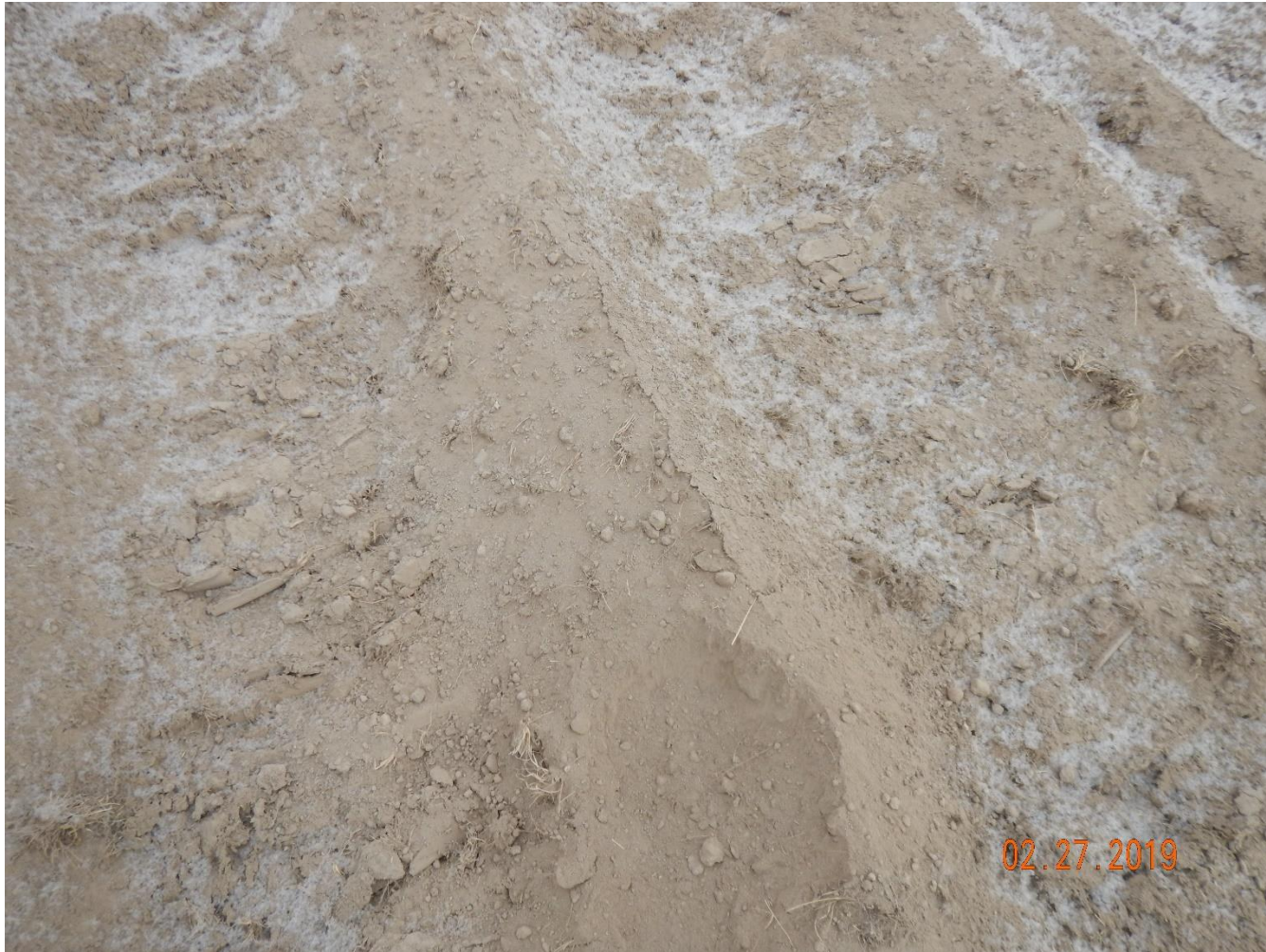
Photo 11: Continued from photo 11. Photo shows tracking does not appear to have been adequate as soils have not been sufficiently stabilized and remain loose material at risk to erosion degradation.
