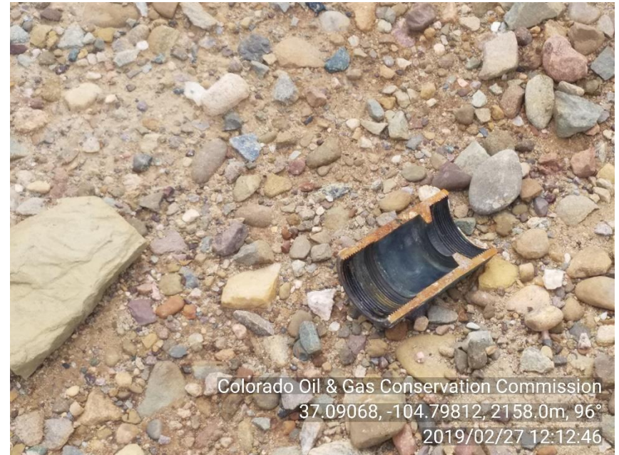
PHOTO 4: HALF OF VALVE ON GROUND UNDER TBG LINE SEPARATION.
