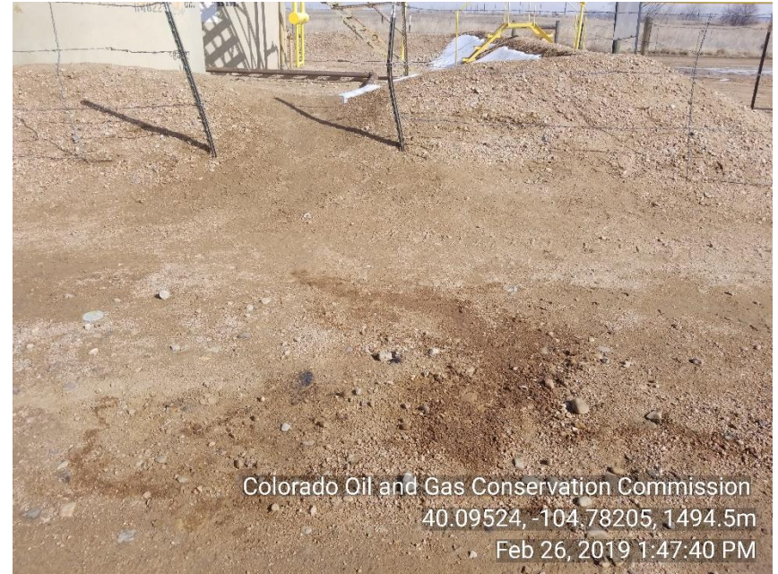
Photo 4 Stained soil appears to be from trucks off loading tanks
