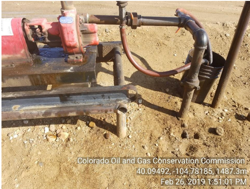
Photo 9 stained soil around recirc pump
