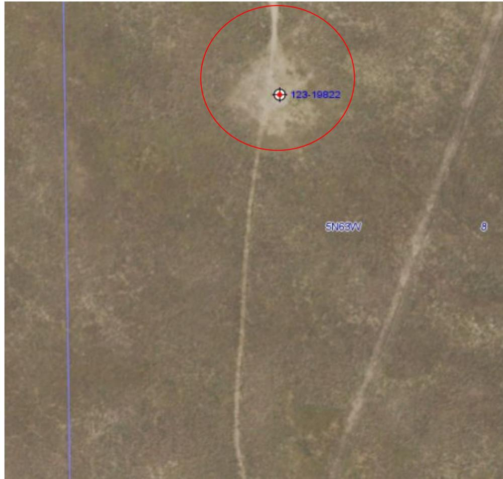
COGCC aerial imagery from 2017 illustrating the Plugged and Abandoned (PA) location (red circle). Operator has failed to perform Final Reclamation at the well location and the associated access road. The offsite tank battery appears to be active and in use for other nearby wells.
