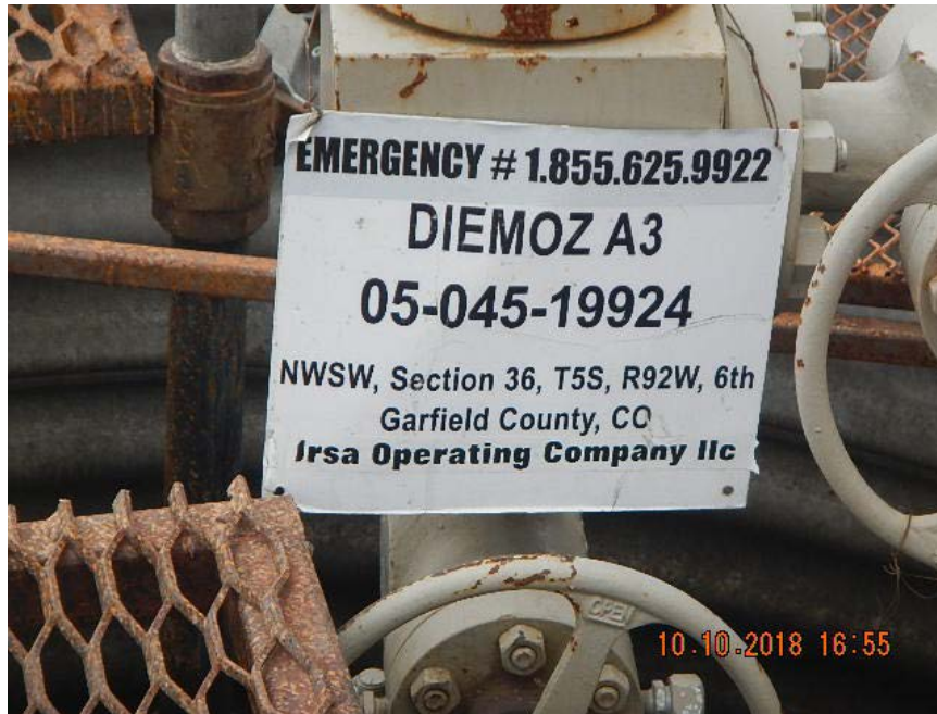
Sign does not meet Rule 210 standards. Photo taken on 10/10/18 FIR # 680200178
