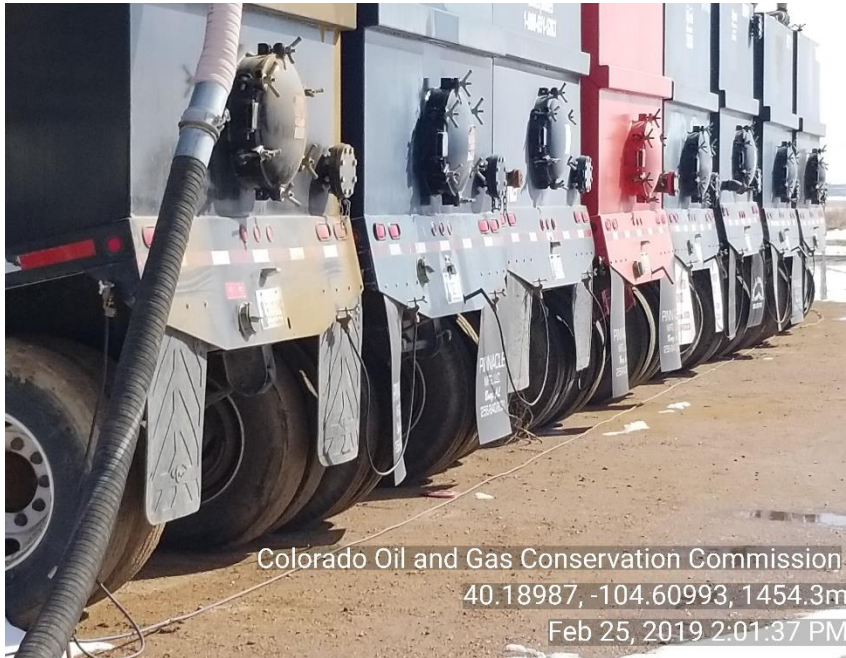
Photo 1 loc pic flow back tanks grounded
