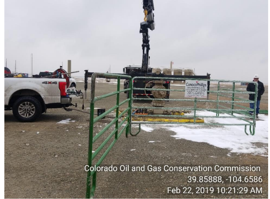
Photo 4WH pic Braden head test all gauges read 0 psi
