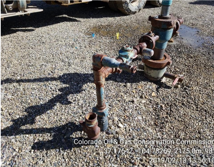
PHOTO 1: WELLHEAD/ UNUNED UNMARKED RIZER NO LO/TO
