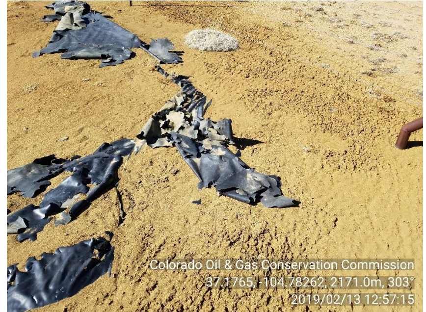
PHOTO 6: PRODUCED WATER PIT LINER IS TORN AND IN DISREPAIR
