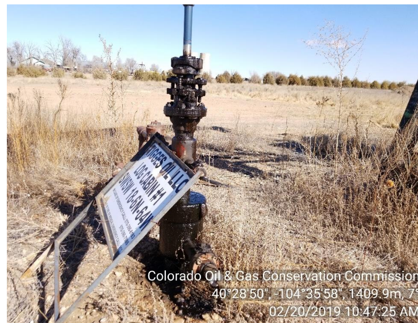
Photo 2: Leaking polish rod from conventional pumping unit
