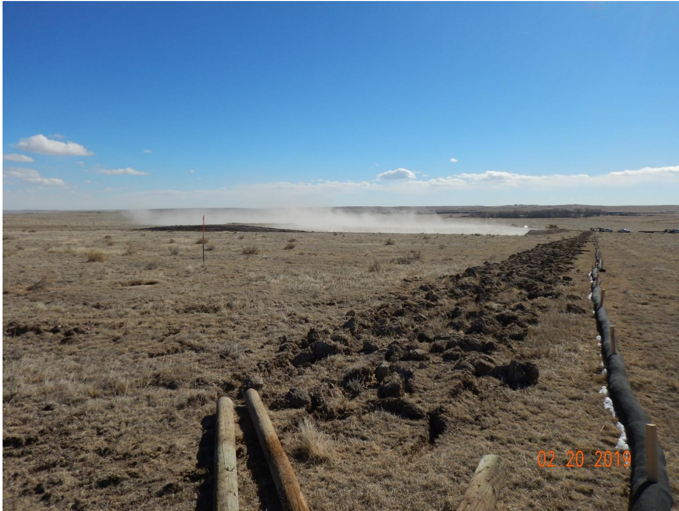
Photo 6: Photo taken from the northwestern area of the disturbance area, facing southeast. Photo shows ongoing wind erosion transporting sediment offsite. This does not comport with rule 1002.e and 1002.f
