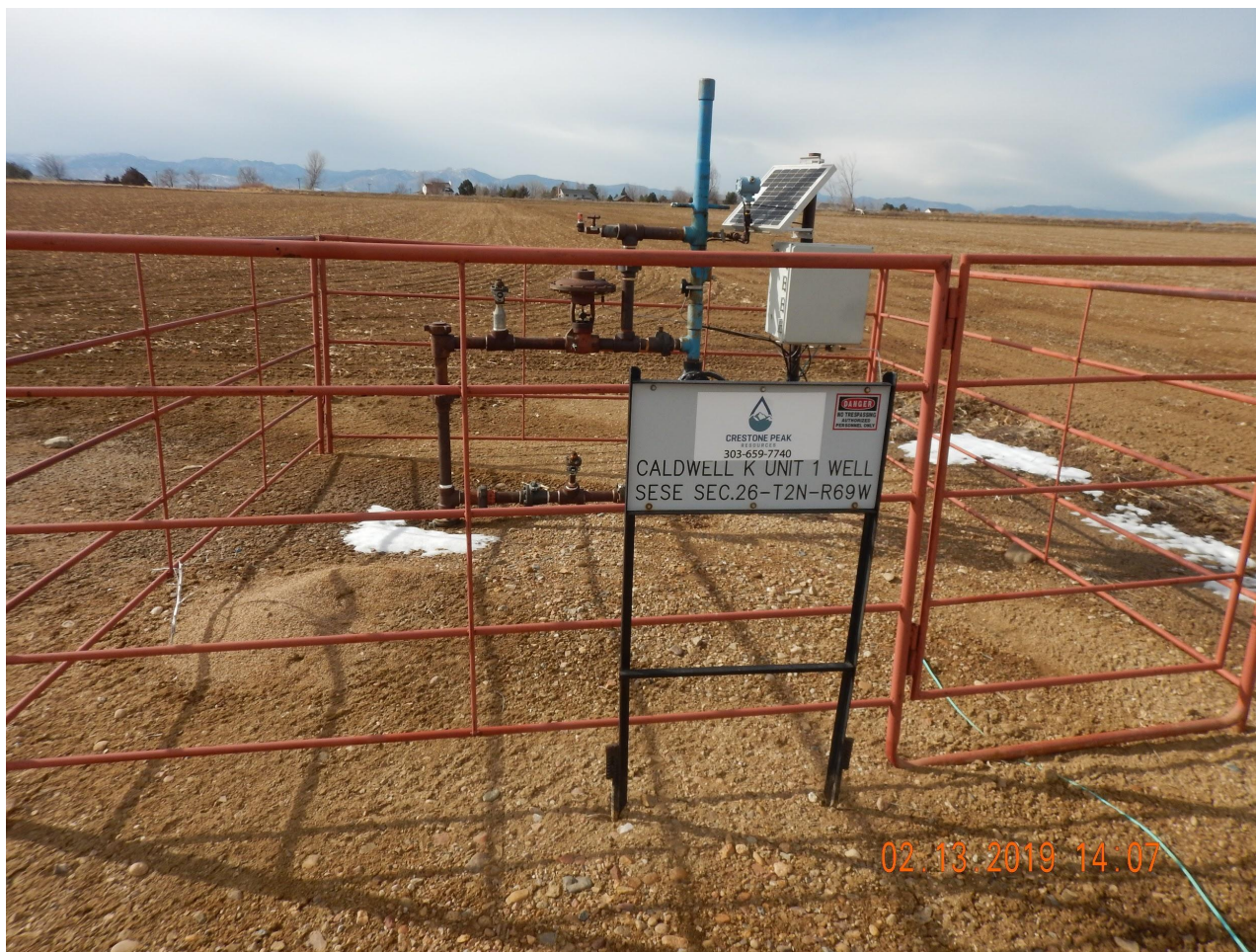
Photo 2. Photo taken from the production/well location, facing West. Photo illustrates only one well was drilled at the location- CALDWELL K UNIT # 1.
