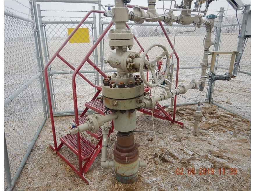
View of (TA) wellhead; flowline has been disconnected.
