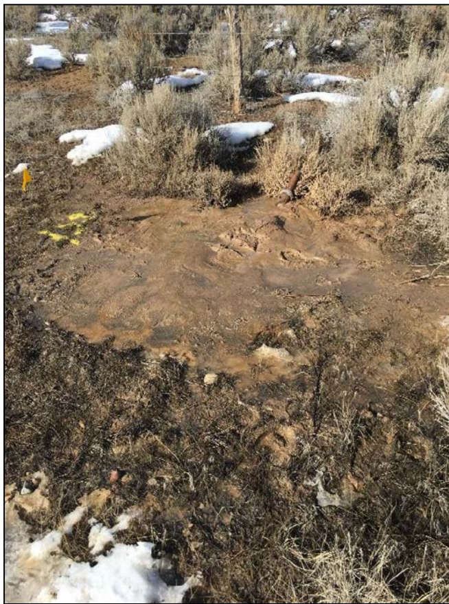
Pipeline leak discovered at the surface
