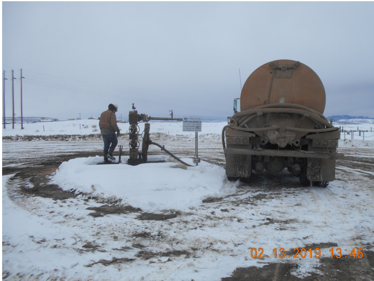
Injection Wellhead
