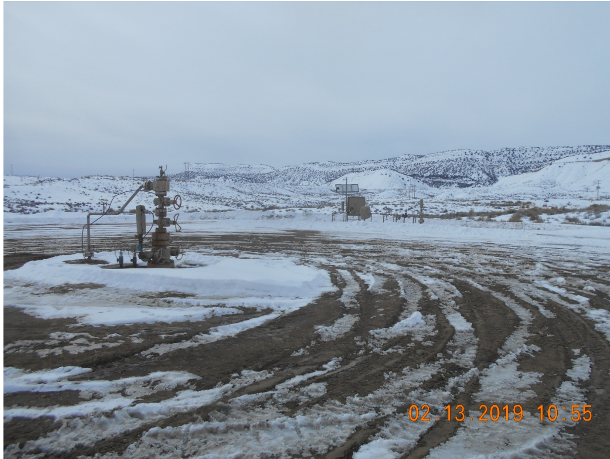
Injection Wellhead
