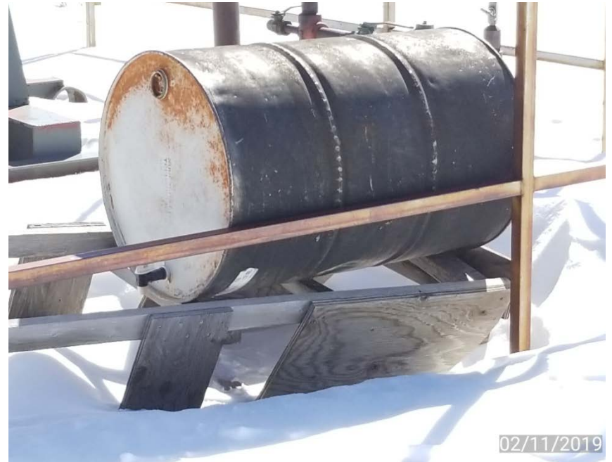
Photo 4. Contents not legible & no secondary containment for barrel.
