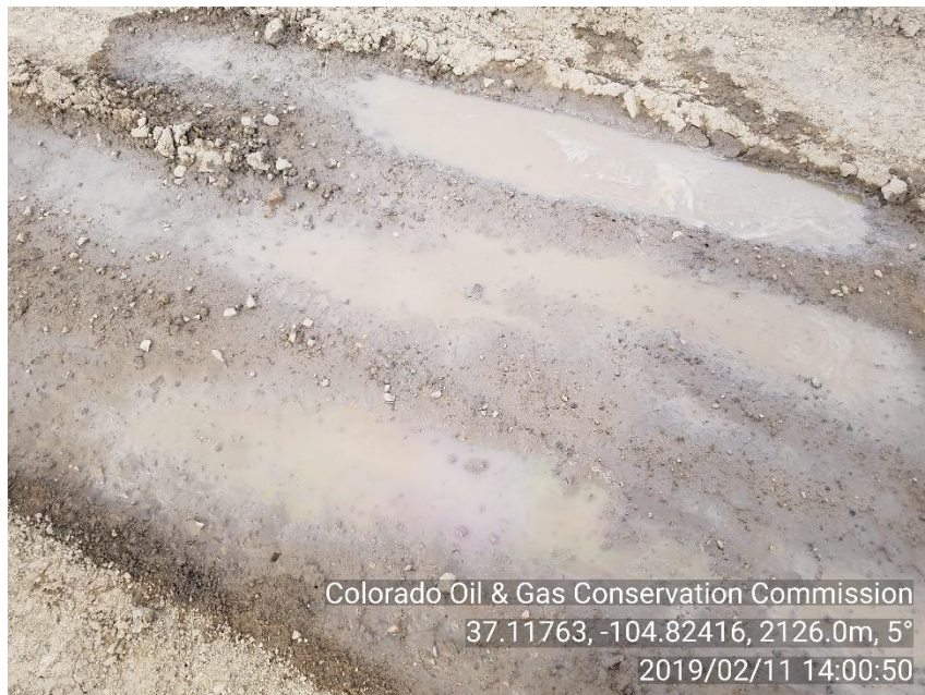
PHOTO 5: RAINBOW SHEEN ON STANDING WATER NEAR GAS METER HOUSE
