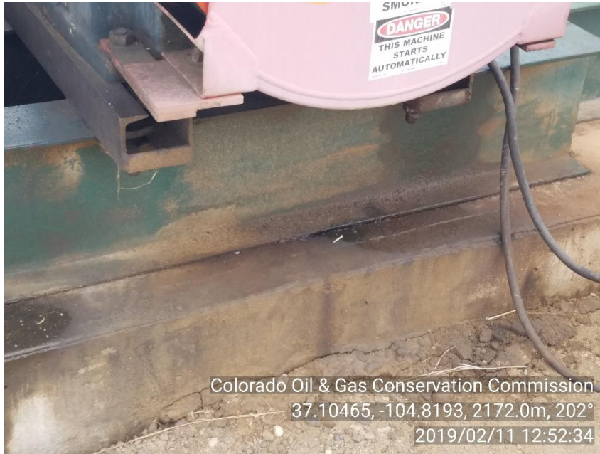
PHOTO 3: STAINED SOIL UNDER GEAR BOX ON PUMP JACK SKID.
