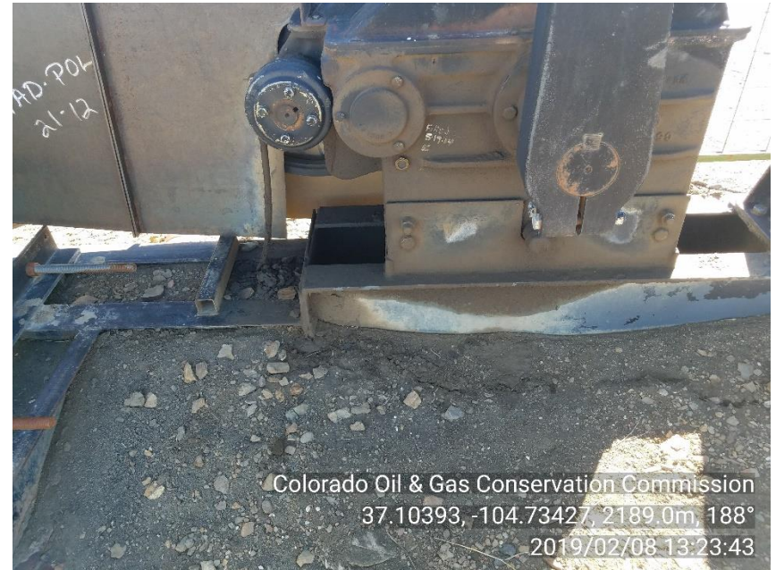
PHOTO 4: STAINED SOIL NEAR PUMP JACK GEAR BOX
