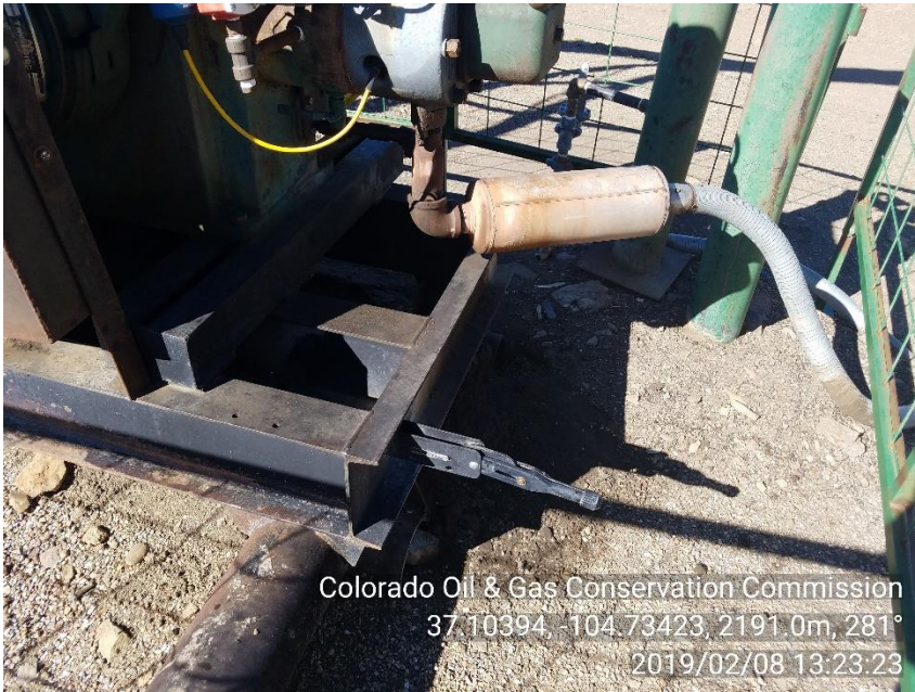
PHOTO 3: STAINED SOIL NEAR PRIME MOVER ON PUMP JACK SKID.
