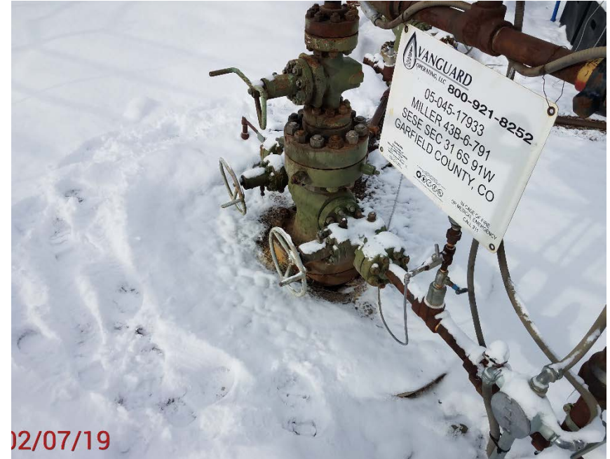
Location Photo #4, Dripping master valve.
