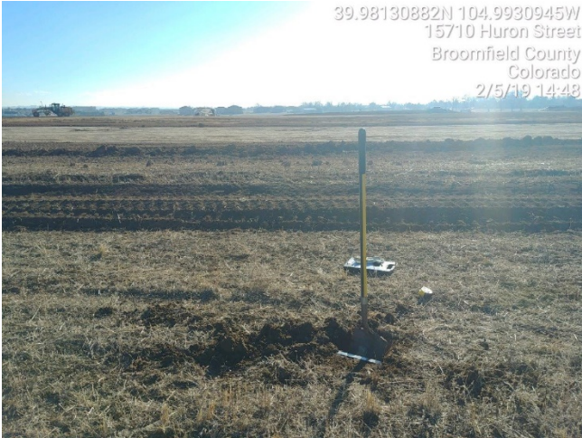
Test Hole #3: The left photo shows the hole is adjacent to the pad disturbance. The top approx. 2" were organic litter and clay. 2-6.5" was a brown clay layer with root structures present. The ruler is placed at the depth the density increased and the shovel was rejected without substantial effort.
