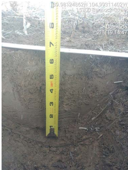
Test Hole #3: The left photo shows the hole is adjacent to the pad disturbance. The top approx. 2" were organic litter and clay. 2-6.5" was a brown clay layer with root structures present. The ruler is placed at the depth the density increased and the shovel was rejected without substantial effort.
