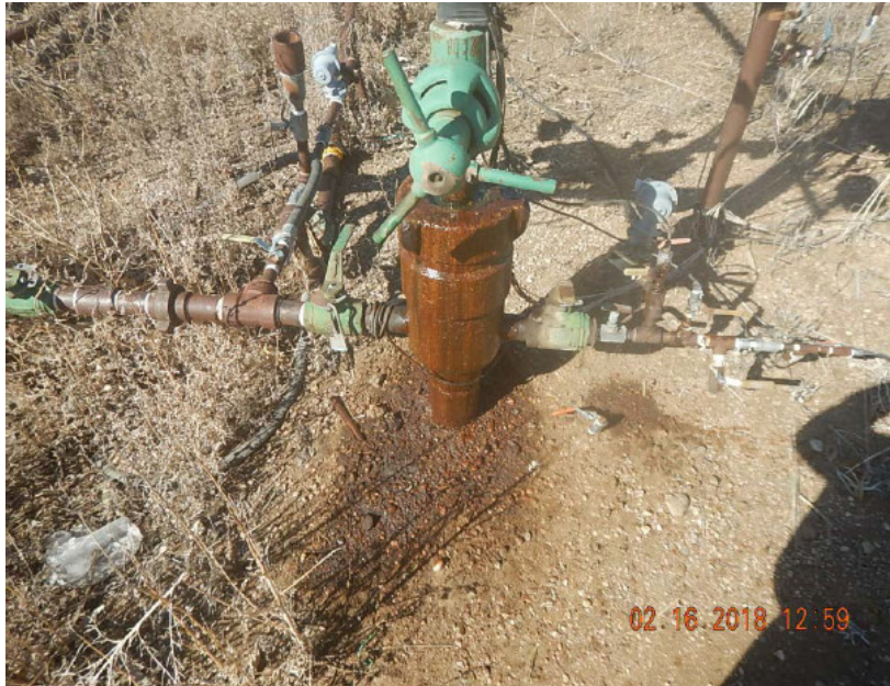
Photo #3 Law 1-17 Wellsite Stained soil & fluids on wellhead from prev. FIR
