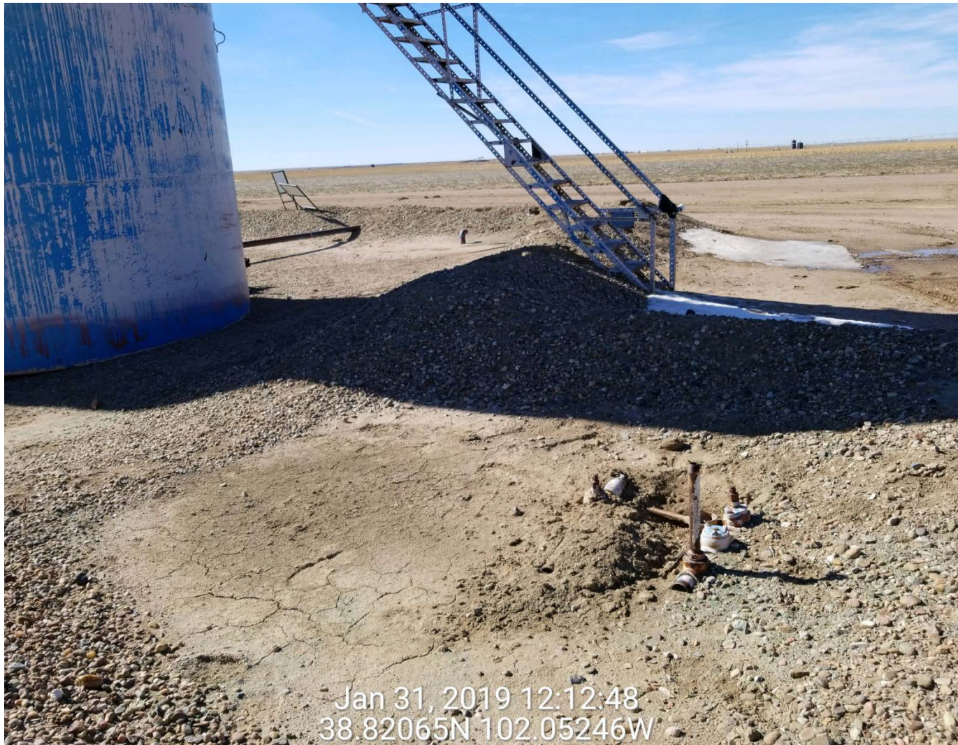
Unmarked pipeline risers
