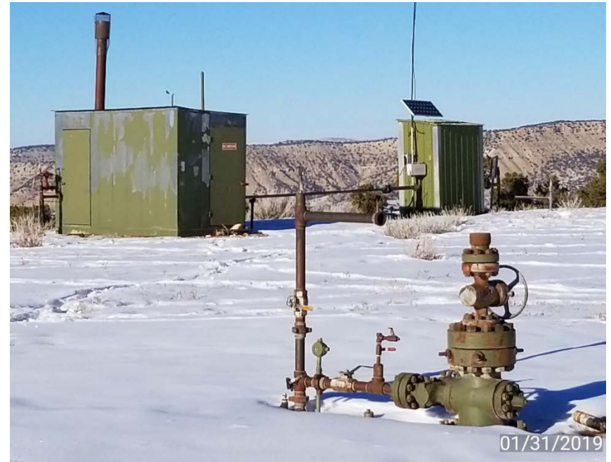
Photo 2. Well head, separator, and meter building.
