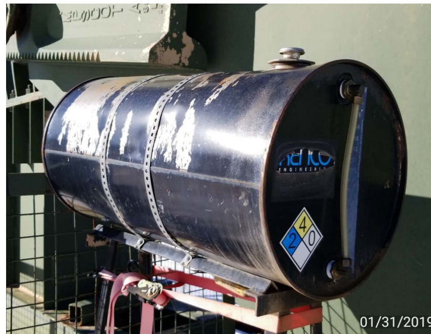
Photo 2. Barrel at pump jack without contents label.
