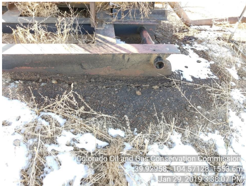
Photo 3 stained soil around PU motor
