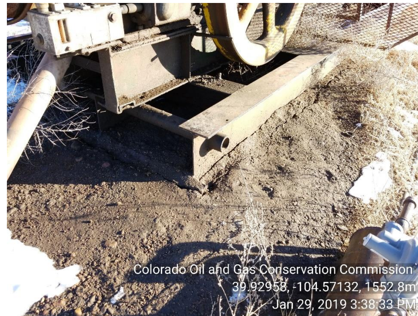
Photo 4 stained soil around PU motor
