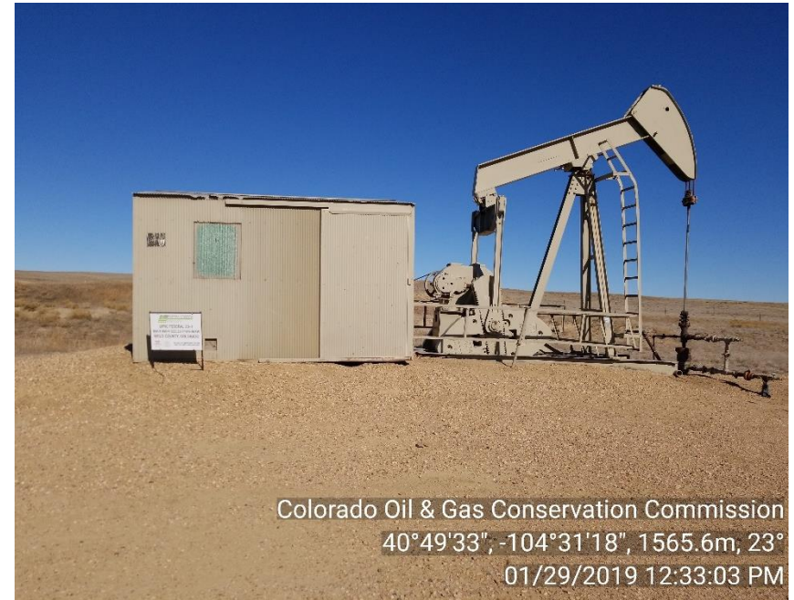
Photo 4: Pump jack with incorrect signage.
