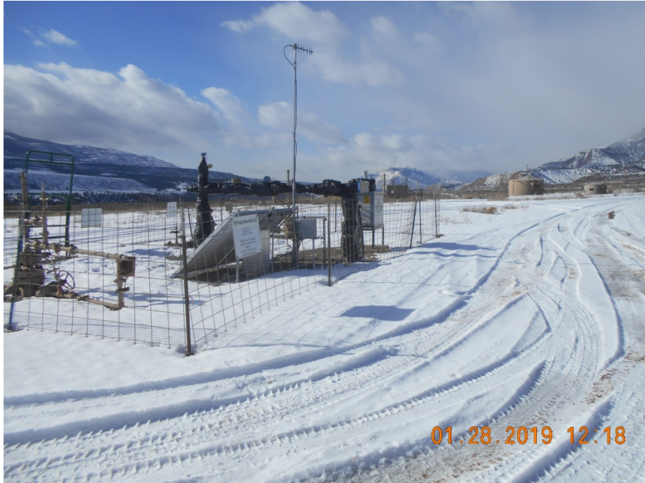
Wellhead with line heater.
